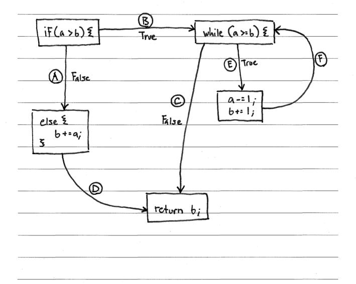
11. [5pts] Fill in the table below with a test suite that provides *path coverage* of the code from the previous question. Cover no more than 2 iterations of the loop. In the covers column, list the relevant labeled items in your CFG that each test case covers. If there is some part of the coverage that is impossible to cover, then list it in the covers column, and put "N/A" in the associated x and y cells. Some cells in the table may be left blank.
