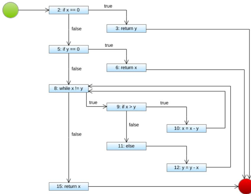
**Statement Coverage:** For each test in the test suite, list the nodes covered by the test case.
