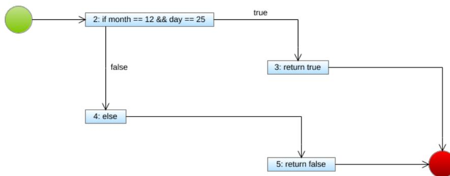
**Statement Coverage:** For each test in the test suite, list the nodes covered by the test case.
