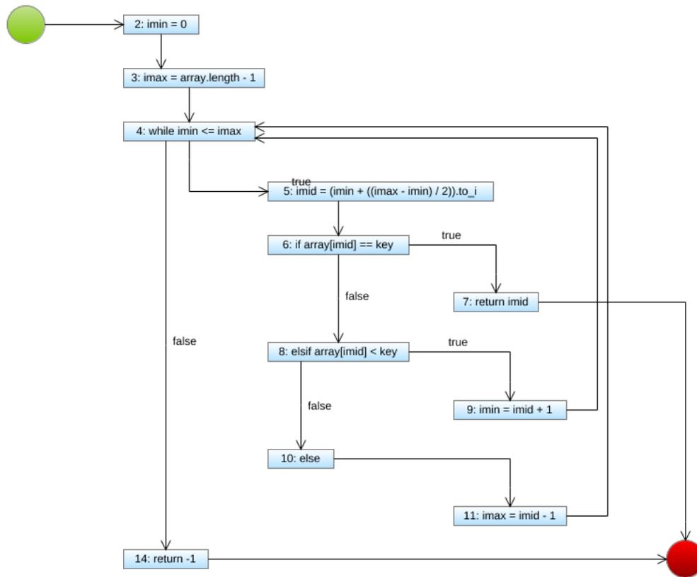
**Statement Coverage:** For each test in the test suite, list the nodes covered by the test case.
