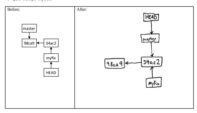
1. Imagine a Git repository ("repo") with one commit and one branch (master). A user makes a new commit to the repo. Draw a box-and-line diagram of the repo like the diagrams shown in class. Include all commit nodes (with made-up hashes), all HEAD nodes, and all branch nodes.
