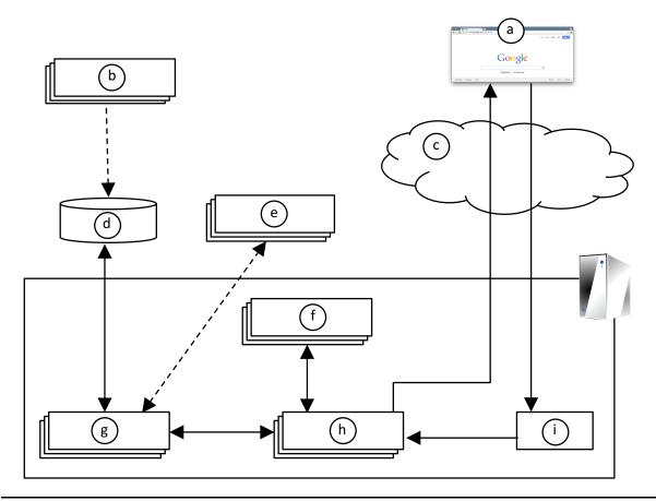
Figure 7. Rails architectural diagram.
